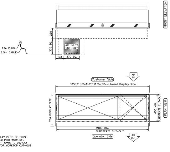
NOTE: IF DISPLAY IS TO BE FLUSH MOUNTED INTO WORKTOP, ADD 4 - 6mm TO DISPLAY SIZES FOR WORKTOP CUT-OUT
